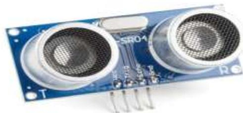
Figure 2 ULTRASONIC SENSOR
